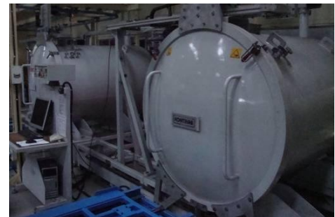
Automatic Gas filling and leakage testing station
